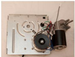
10. Grasp the RPM reader and remove. Take special care not to damage the RPM reader as the teeth are easily damaged.
