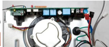
6. Remove all of the five wire connections (A-E) connected to the logic board. Connections A & B will pull directly off. Connections C, D, & E require you to press & release a clip located on the bottom of each connector. Once the clip is pressed, remove the connection.
