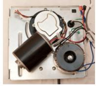
8. Flip the opener chassis over. Using a 10mm wrench remove the three bolts securing the motor and RPM reader. While holding the motor and chassis carefully flip opener chassis back over.
