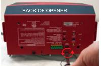
4. Using a Phillips screwdriver remove the four screws securing the bottom of the plastic motor cover.
