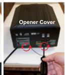
5. Using a Phillips screwdriver remove the six screws securing the bottom of plastic motor cover.
