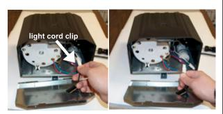
4. Unplug the light cord by pressing down on the light cord clip & separating the connectors. Remove the metal light cover.
