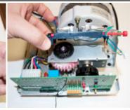
7. Remove the limit system assembly. First remove the limit wire from the logic board. Second push in the three tabs with your finger until you feel them disengage. Finish by pulling up gently on the limit system assembly to disengage.
