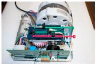
6. Remove the opener cover from the base unit. It is EXTREMELY important not to damage the open, close and learn buttons. Grasp the front of the cover (as pictured) and pull up and back on the cover to remove. Remove the remote wire from the opener cover. Finish by removing the opener cover.
