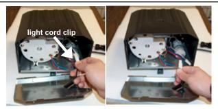
4. Unplug the light cord by pressing down on the light cord clip & separating the connectors. Remove the metal light cover.
