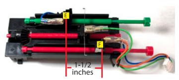
7. If properly adjusted Close limit stop (F) and Open limit stop (E) should be exactly 1-1/2 inches apart.
