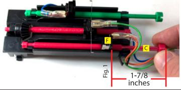
5. Adjust the close limit screw (C) by turning it either clockwise or counter clockwise until the close limit stop (F) is set according to the measurements shown in figure 1.
