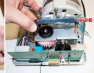
3. Remove the limit system assembly. First remove the limit wire from the logic board. Second push in the three tabs with your finger until you feel them disengage. Finish by pulling up gently on the limit system assembly to disengage.
