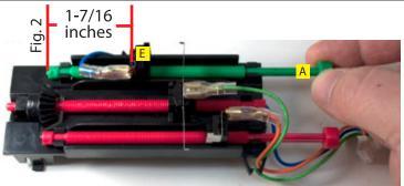
6 . Adjust the open limit screw (A) by turning it either clockwise or counter clockwise until the open limit stop (E) is set according to the measurements shown in figure 2.
