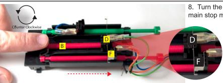
8. Turn the main limit travel screw (B) counter clockwise until the main stop module lightly touches the close limit stop (F)
